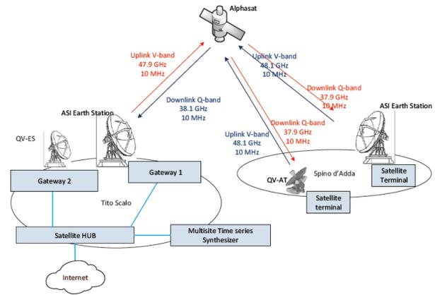
Fig. 2 shows the main components of the test scenario:
